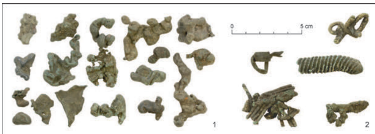
Fig. 6. Demänovská hora site. Melted amorphous bronze lumps and heavily burnt and melted together fragments of bronze objects. Photo by P. Červen.
