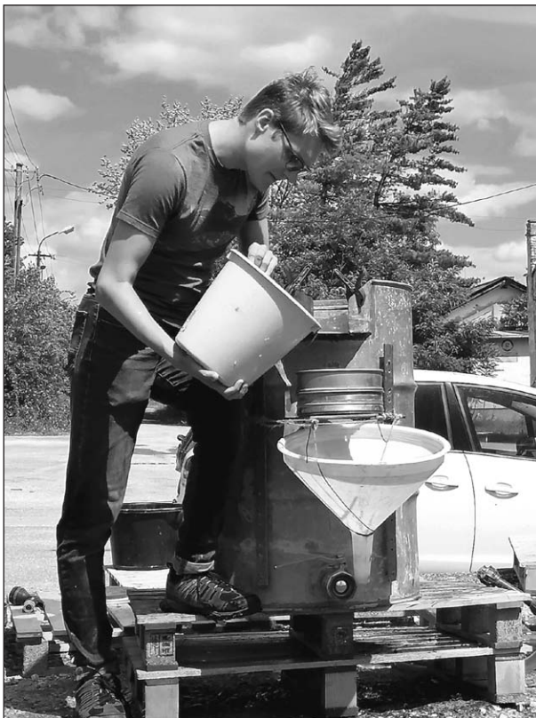
Fig. 2. Manual wash-over processing of heavy fraction using a bucket system.
